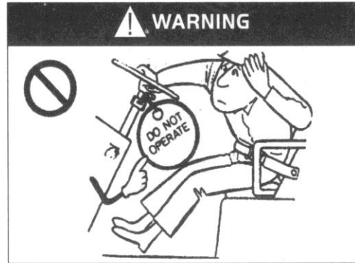
Do not drive an unsafe forklift!
